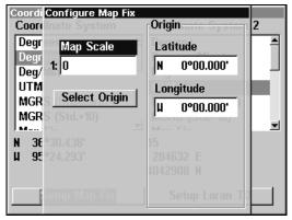
Configure a map fix so the unit can find your position on a printed chart or topographical map.
